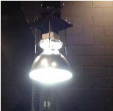
Fi8550A luminaire mounted on goniometer.
